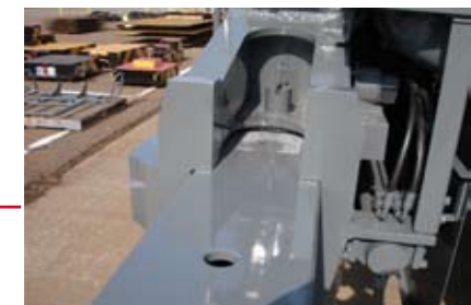
Outrigger lock pins Outrigger extension potentiometer.
