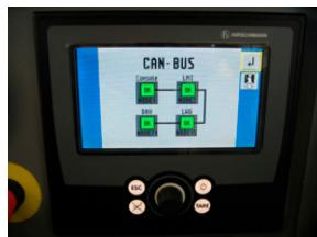
• **Full CAN-Bus:** Simplifies troubleshooting, reduces down time, allows high speed data transfer and real time diagnosis. Software based allows for customization of functions and troubleshooting from a laptop computer.
