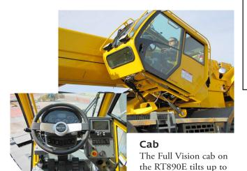
20° providing the operator additional comfort when working at long boom and
