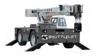
Standard: 41 ft. (12.5m) main boom on the 5540F 54 ft. 6 in. (16.6m) main boom on the 5560B Optional: 5540F: Manual 4th main boom section adds
