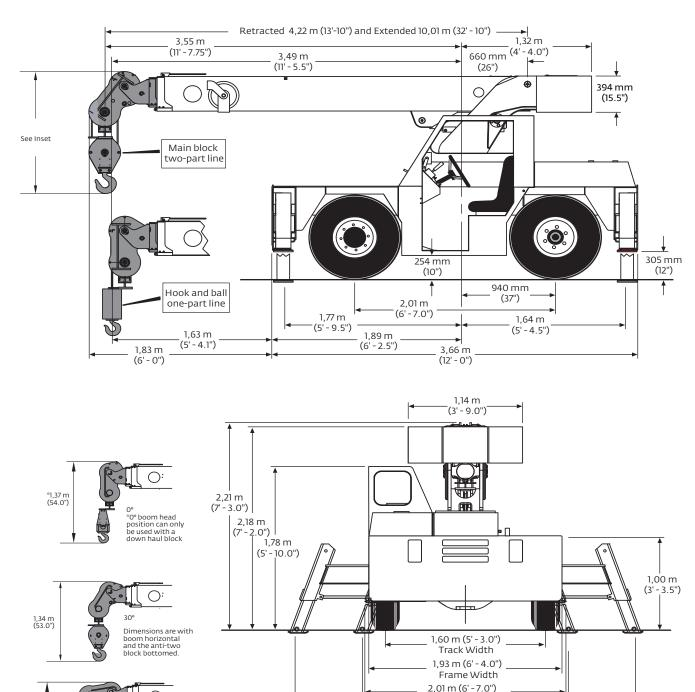
Dimensions are with boom horizontal and the anti-two block bottomed.
