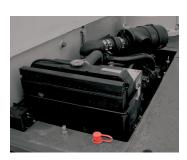
Engine (Tier IV) Standard: Cummins QSB 3.3 L turbo-charged diesel rated at 74,5 kW (100 bhp) at 2600 rpm.
