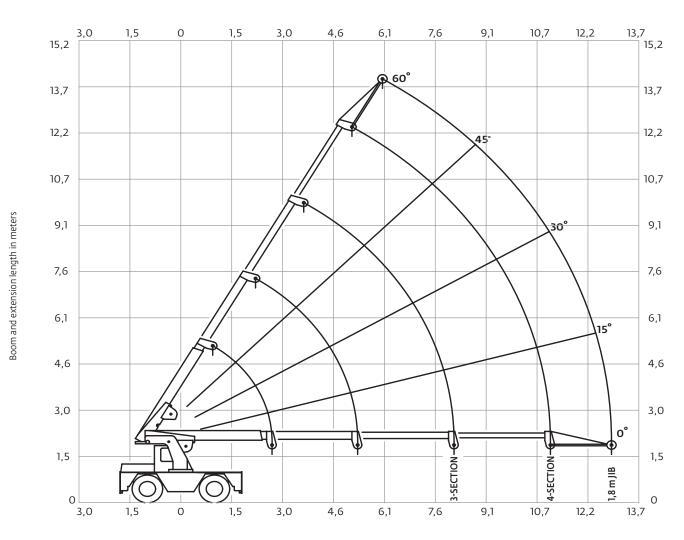
Operating radius in meters from axis of rotation  $% \left( 1\right) =\left( 1\right) \left( 1$
