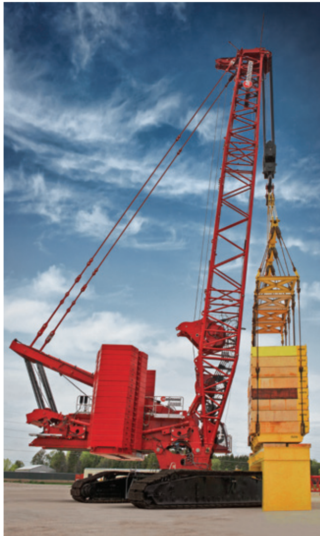
The MLC650 effortlessly lifts 650 t (717 USt) of test weights to certify its advertised capacity.
