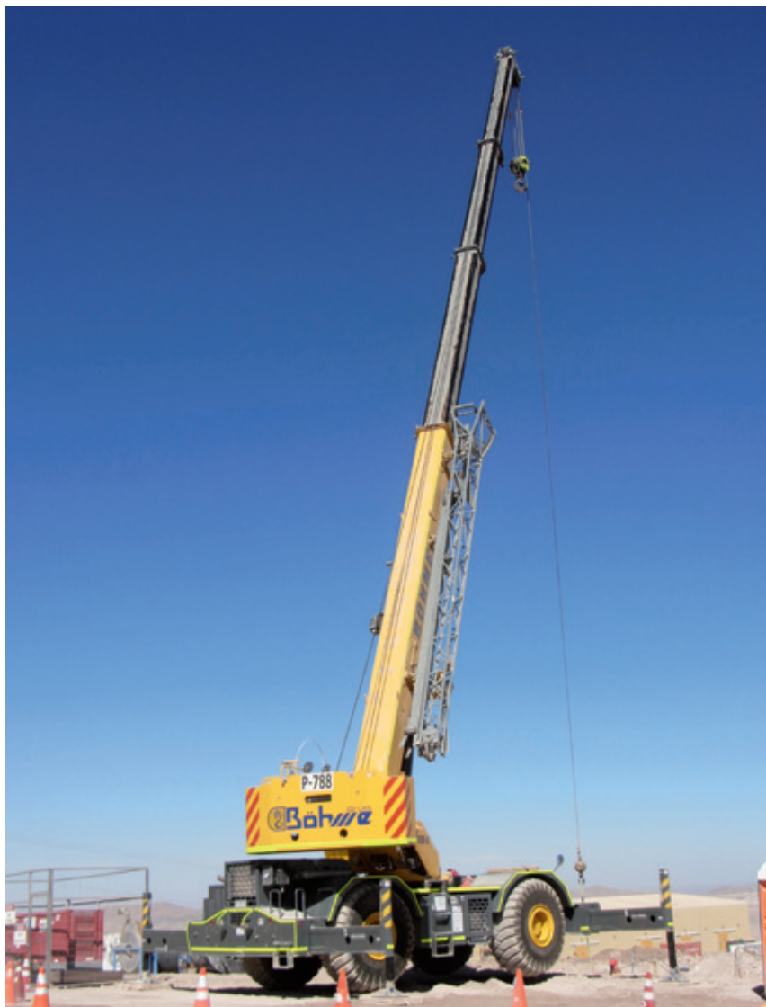
The Grove RT765E-2 takes care of most of the day-to-day lifting jobs at the Sierra Gorda mine.
